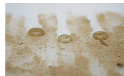
Fig.3 anti dirt and self-cleaning function of water droplets
